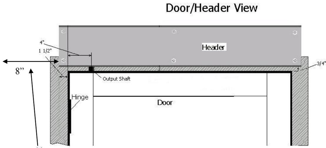
**NOTE:** If door is an In-Swing, allow 8” minimum between header and opposing wall to allow clearance for the Pull Arm.
