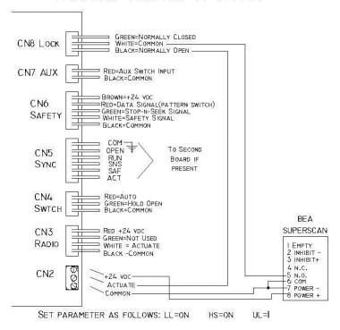
Wire the Super Scan to the ACTUATE input instead of the AUX input and put the normally open side of the lock relay in series with it. (I am assuming since the door can be used manually, there's no lock. This won't work without an extra relay and more wiring hassle if the lock relay contacts are already in use to operate a lock).
