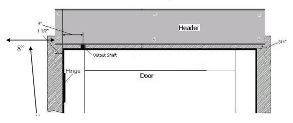
**NOTE:** If door is an In-Swing, allow 8" minimum between header and opposing wall to allow clearance for the Pull Arm.
